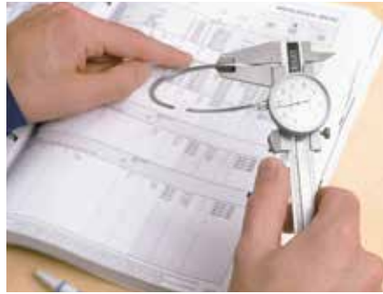
Checking with KS calliper with dial gauge, accuracy 0.01 mm KS art. no. 50 009 814
