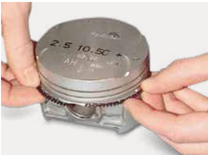
1. The expander spring is fitted into the groove.
