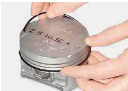
2. The bottom fin is inserted by 120° joint twist.
