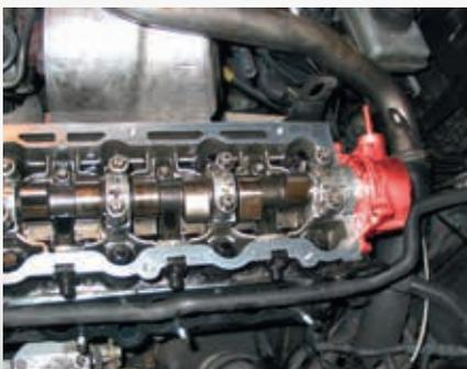
*The state of the art is represented by single-vane vacuum pumps which are driven by the camshaft.*
