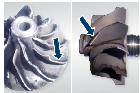
ill. 4: Casing of compressor wheel (left) and turbine wheel (right) damaged symmetrically as a result of friction on the casings
