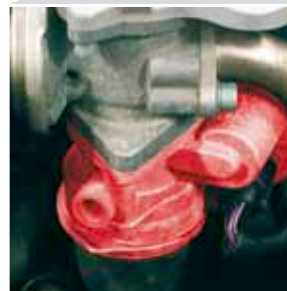
Close-up view of the regulating throttle (emphasised in red)
