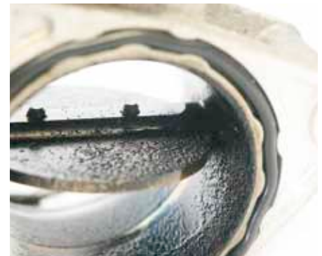
Regulating throttle suffering from oil contamination
