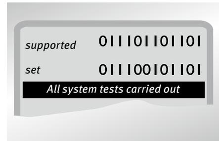
Fig. 4: readiness code after successful test (example)
