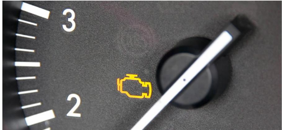
Fig. 6: malfunction indicator lamp (MIL)
