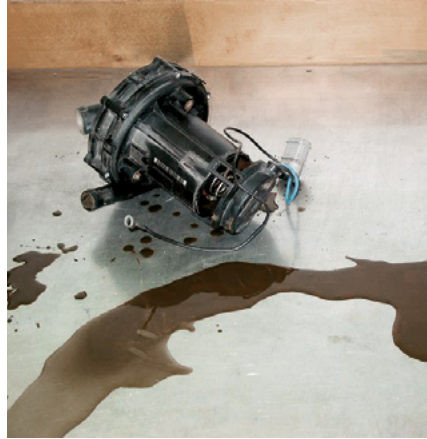
Fig. 28: condensate in the secondary air pump
