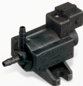
Solenoid switching valves act as switches for vacuum-controlled components. They are required for opening and closing pneumatic secondary air valves.
