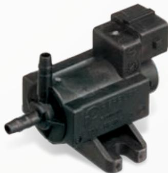
Solenoid switching valves act as switches for vacuum-controlled components. They are required for opening and closing pneumatic secondary-air valves. The latest generation of secondary-air valves manages without actuation by a solenoid switching valve.
