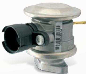
The shut-off function ensures that secondary-air is only routed to the exhaust manifold in the cold starting phase. The integrated non-return function stops exhaust gas, condensate or pressure peaks in the exhaust system (e.g. misfiring) causing damage to the secondary-air pump.
