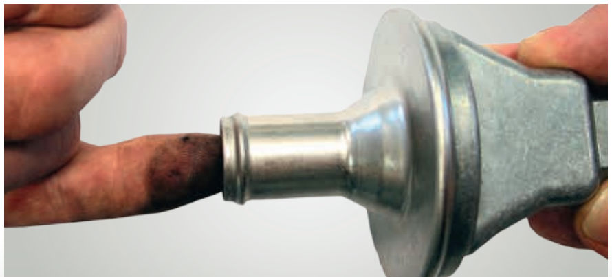
Fig. 1: Simple inspection of the non-return valve
