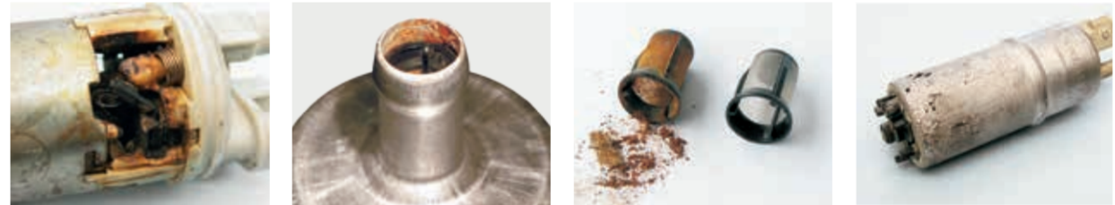
Scorching due to dry running Rusted pump inlet (water damage) Blocked sieve filter and new condition Contact corrosion
