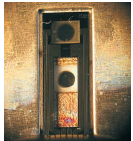
Right: In this case, there is hardly any film left. The sensor looks "sandblasted".
