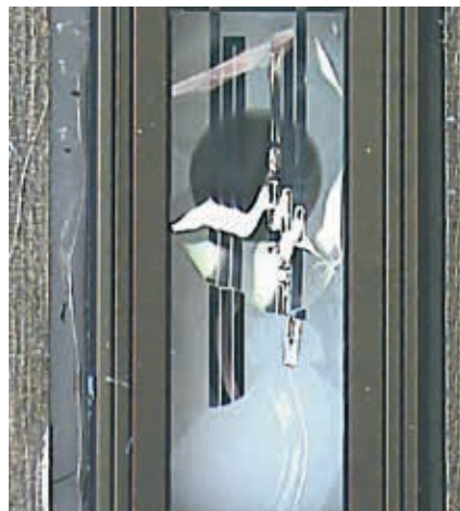
Left: The film to which the sensor elements are applied has been "bombarded" by particles.
