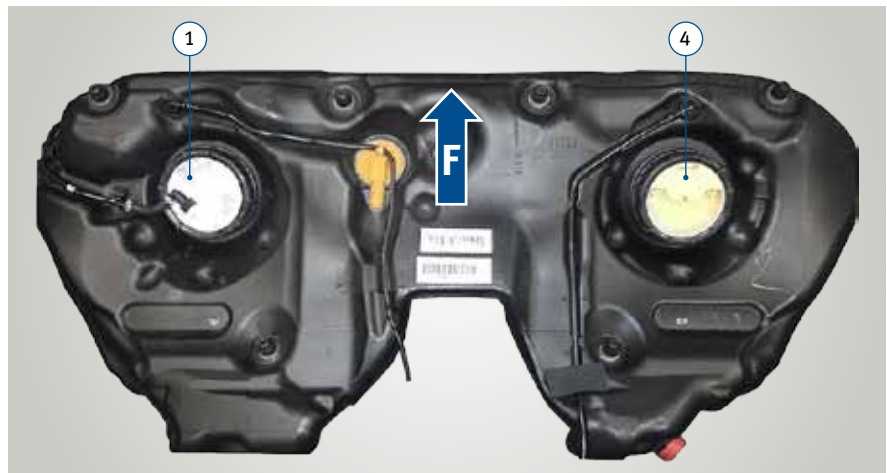
Fig. 4: Fuel tank (top-down view)
