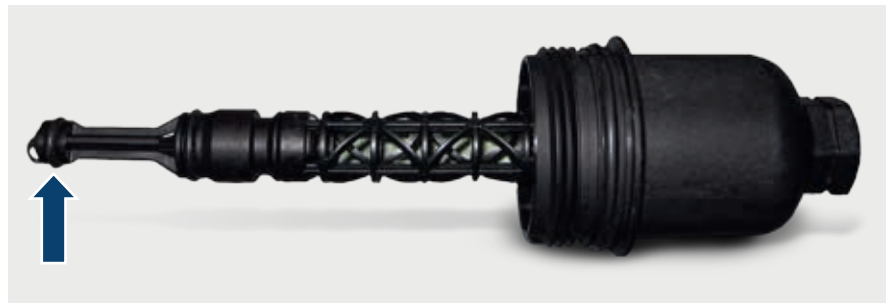
Fig. 1: Plastic tube at the oil filter cap (MB OM611, OM646, M271) Detail: Drainage valve seal – keeper with sealing ring
