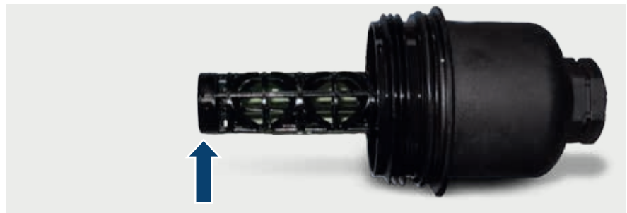
Fig. 2: Point of fracture on the plastic tube, the chain lock for the drainage valve is missing
