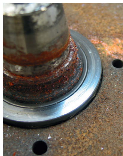
Destroyed sliding ring seal – the sliding surface was corroded by foreign particles
