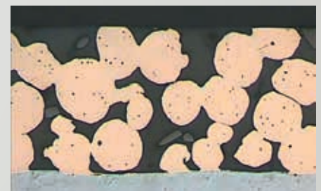
Fig. 4: Condition at end of running-in process. The bronze layer begins to function.
