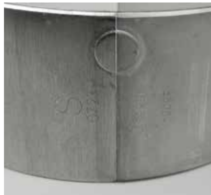
Locking lugs of the OE engine bearing shells. This shape, which is also known as "moon version", is also protected by patent.
