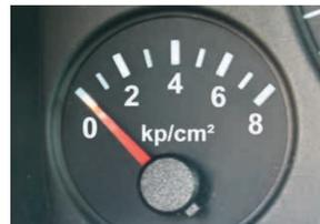
Insufficient oil pressure leads to premature wear of the bearings or to bearing damage. The main reasons for this are:
