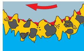
Impurities in the engine oil such as dirt, abrasion, coolant and fuel lead to the oil losing its lubricating effect. Either solid parts cause mixed friction to start or the viscosity of the lubricating oil is reduced by other impurities in liquid form until the oil can no longer perform its support function within the bearing and the lubricating film is separated. The resulting mixed friction leads to rapid wear and destruction of the bearing.
