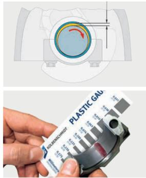
The bearing clearance ensures that in every operating situation there is sufficient space between the bearing and the bearing journal. This enables a strong and stable film of oil to form and pure liquid friction is possible.
