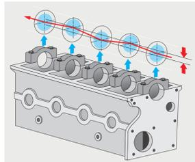
If the centre points of all main bearing points are not exactly central on an axis, severe bearing damage occurs when starting due to the necessary bearing clearance being eliminated. Such problems are caused by bent or incorrectly ground crankshafts and a distorted engine case (previous damage caused by overheating).
