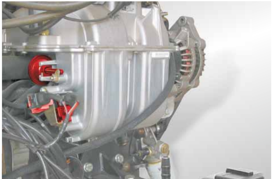
At the controlled intake manifold in the Opel Astra already two EUVs have been fitted (highlighted in red). One controls through the actuator above it (highlighted in red) the intake manifold throttles; the other switches the secondary air shut-off valve (not shown)
