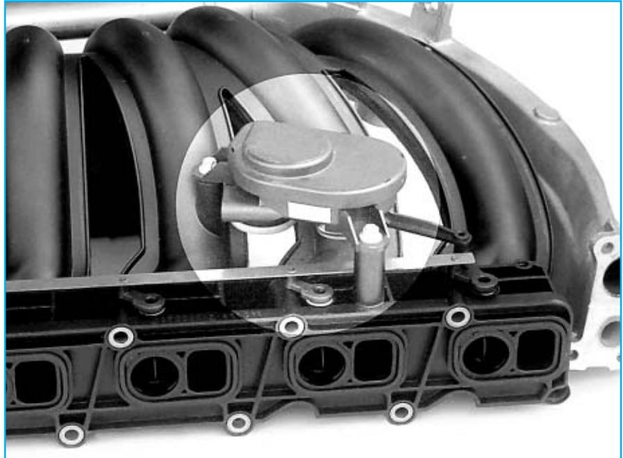
Intake pipe with EDM-i (highlighted)
