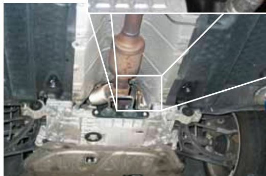
Bypass valve in VW EOS TFSI (highlighted in red)
