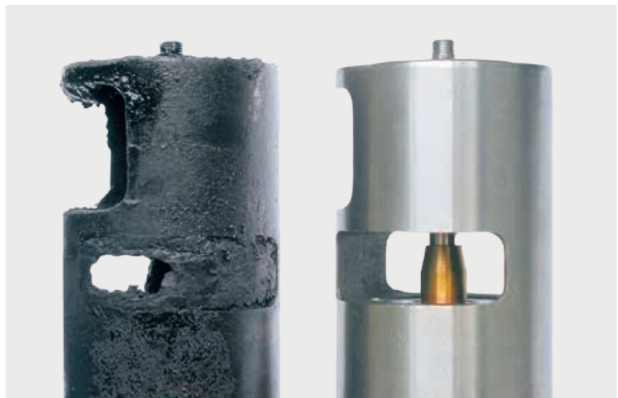
EGR valve with sticky deposits and EGR valve as new
