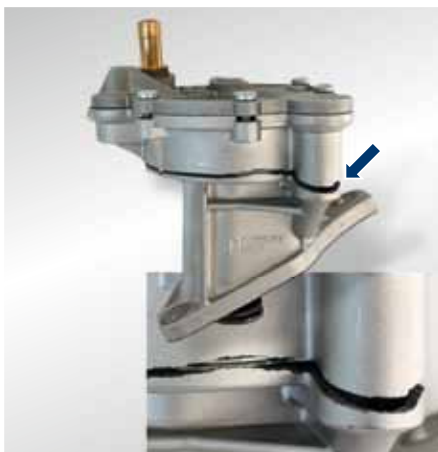
Fig. 1: Broken pump casing
