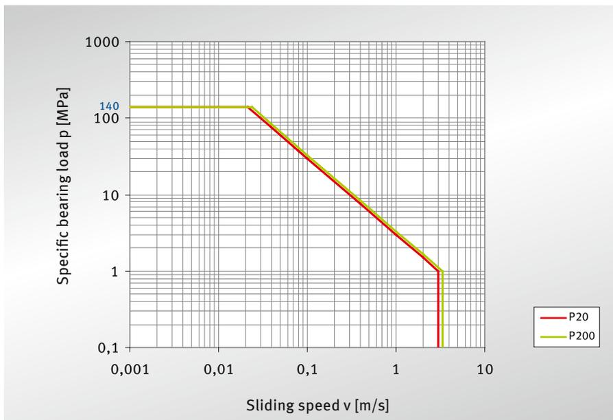
Fig. 3: pv value [MPa·m/s], limit curve (values apply at room temperature)
