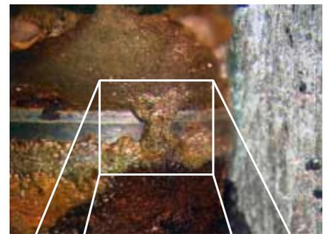
Fig. 5: Corroded sealing seat
