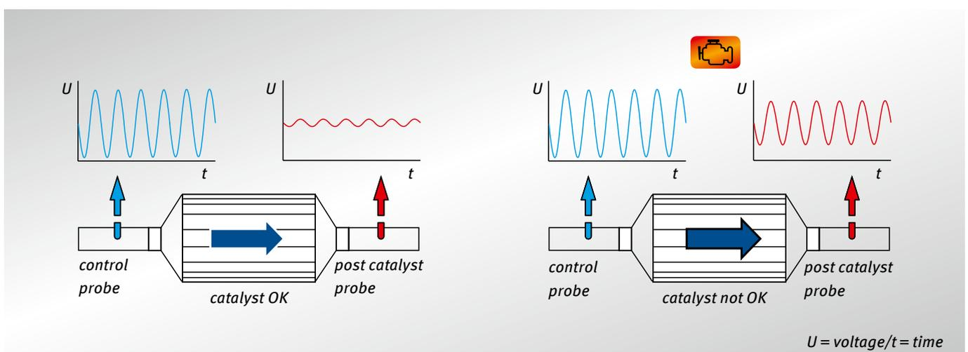
Fig. 45: monitoring the efficiency of the catalytic converter
