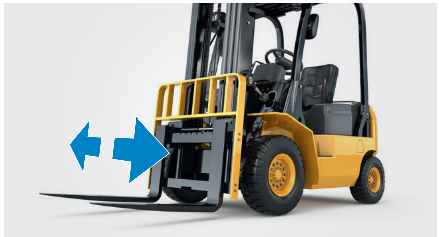
Guidance of the fork lateral adjustment
