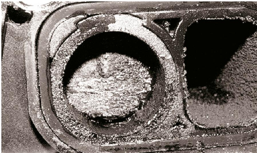
Fig. 44: tumble flaps, malfunction due to heavy deposits
