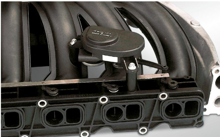
Fig. 41: intake manifold with tumble flaps and EAM-i
