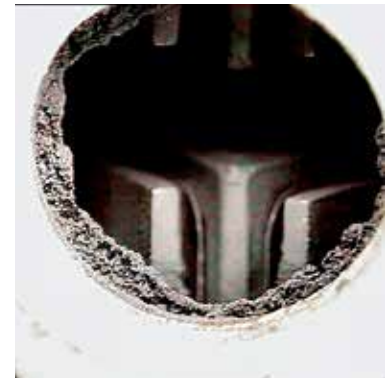
示意图31: 止回阀内的废渣沉积
