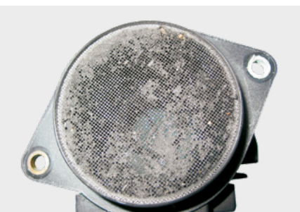
Blocked air mass sensor (LMS)
