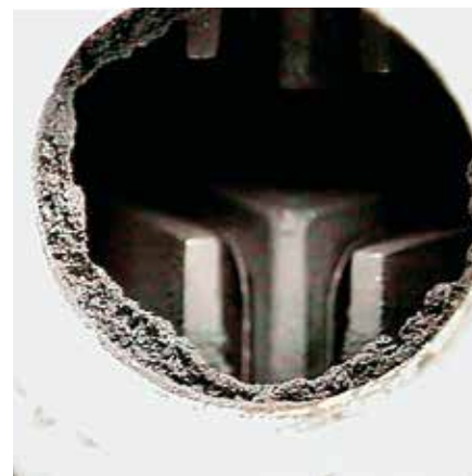
Fig. 31: deposits in the non-return valve
