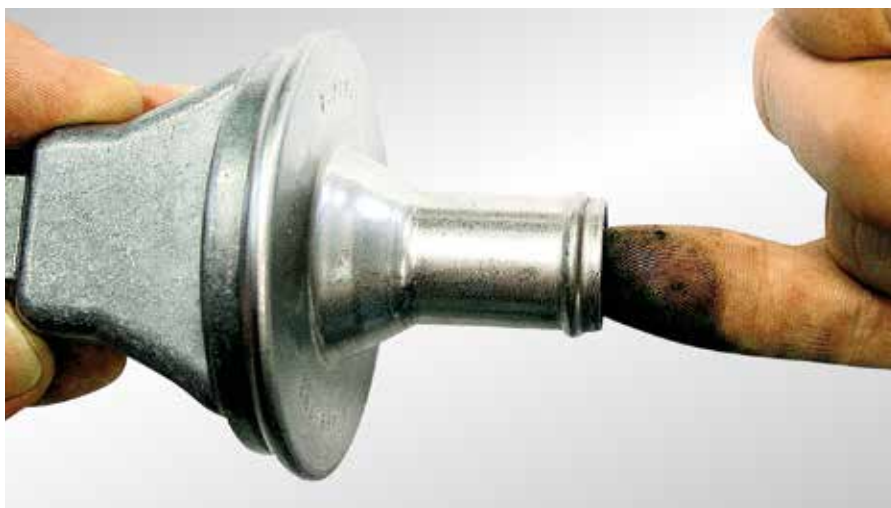
Fig. 32: simple check of the check valve
