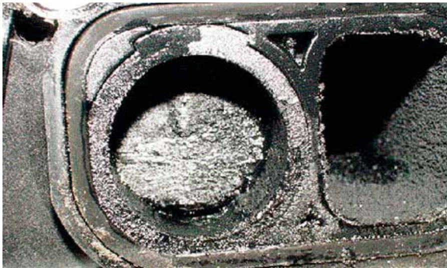
Fig. 44: tumble flaps, malfunction due to heavy deposits
