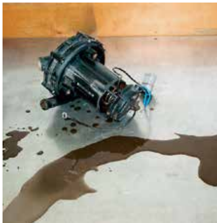
Fig. 28: condensate in the secondary air pump
