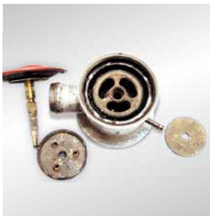
Fig. 30: cut-off secondary air valve – damage to the diaphragm and valve plate due to condensates
