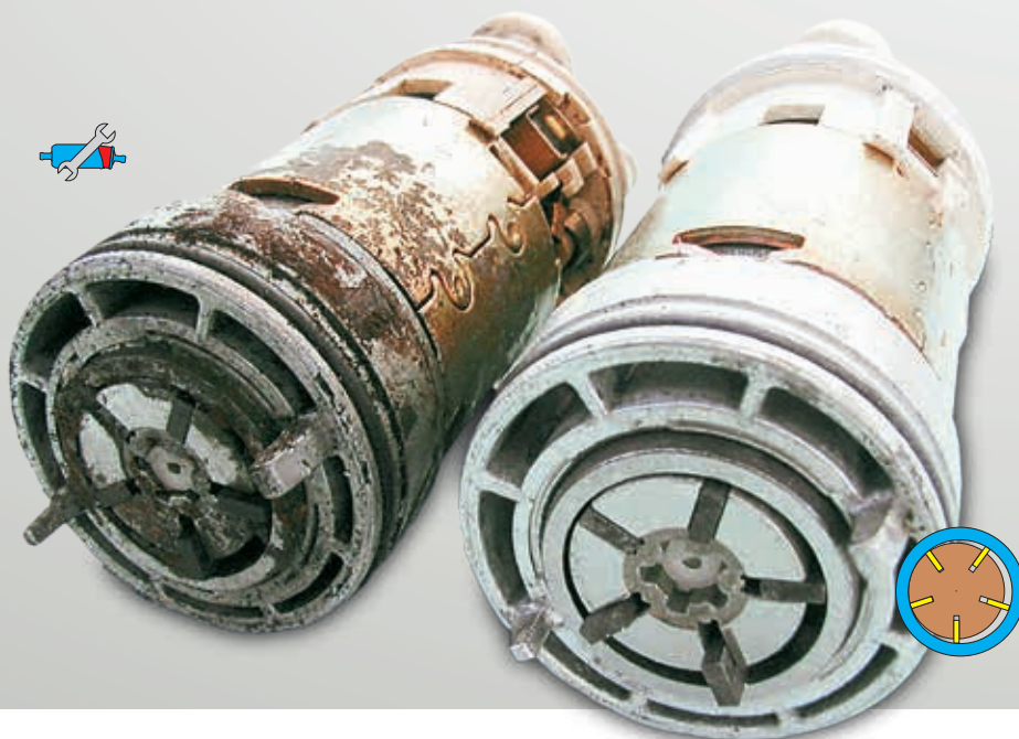
Fig. 36: Water damage to a vane-type pump On the right for the purpose of comparison is a fuel pump with comparable mileage, which has not been exposed to water.
