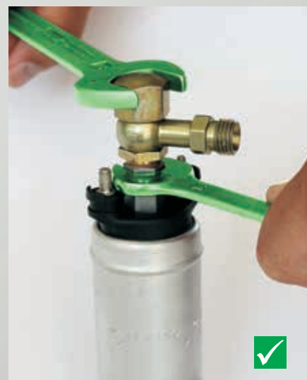
Fig. 71: Correct installation: The lower hex nut of the fuel pump must be counter-tightened
