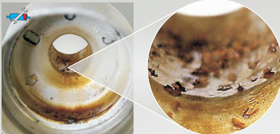
Fig. 64: Crystalline deposits caused by unsuitable fluids
