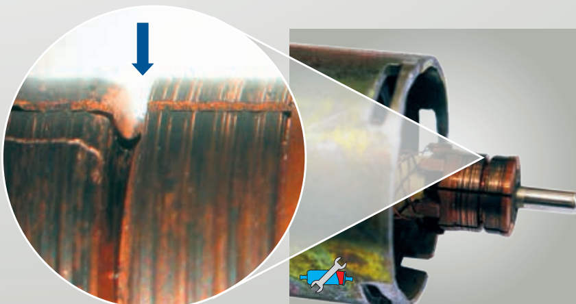
Fig. 63: Destroyed glide path of pole changer
