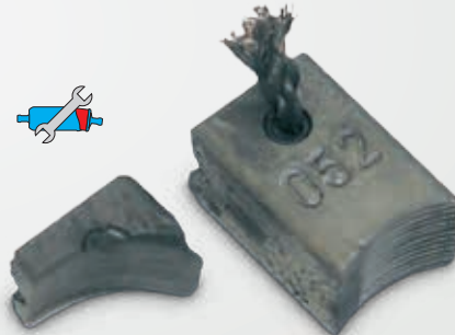
Fig. 62: Sliding contacts at approx. 9,500 miles
