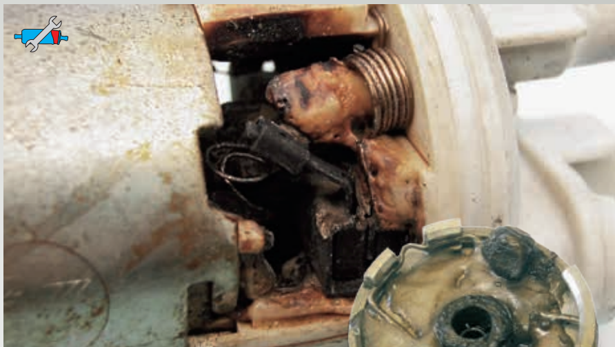
Fig. 20: Friction welding caused by dry running
