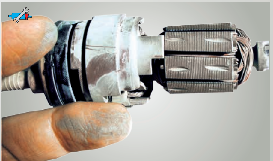
Fig. 56: Coating from poor-quality fuel
