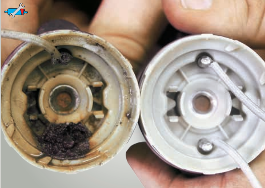
Fig. 46: Left: Corroded electrical contacts. Right: New condition
