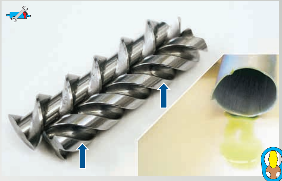
Fig. 55: Adhesion due to a non-compliant fluid
