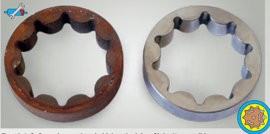
Fig. 48: Left: Severely rusted trochoidal toothed ring. Right: New condition
