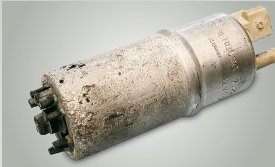
Fig. 72: Contact corrosion due to incorrect material combination
