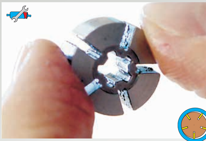
Fig. 30: Contaminated pump system of a vane-type pump
