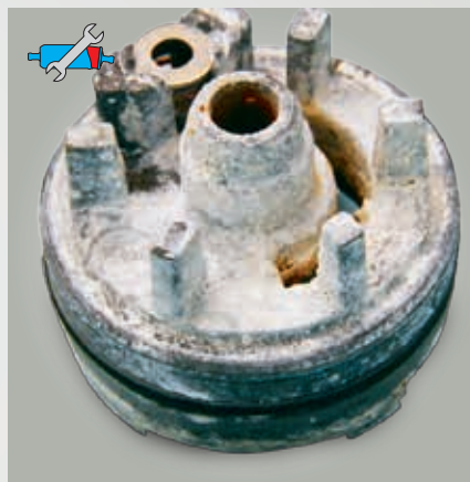
Fig. 50: Calcified outer bearing of a fuel pump
