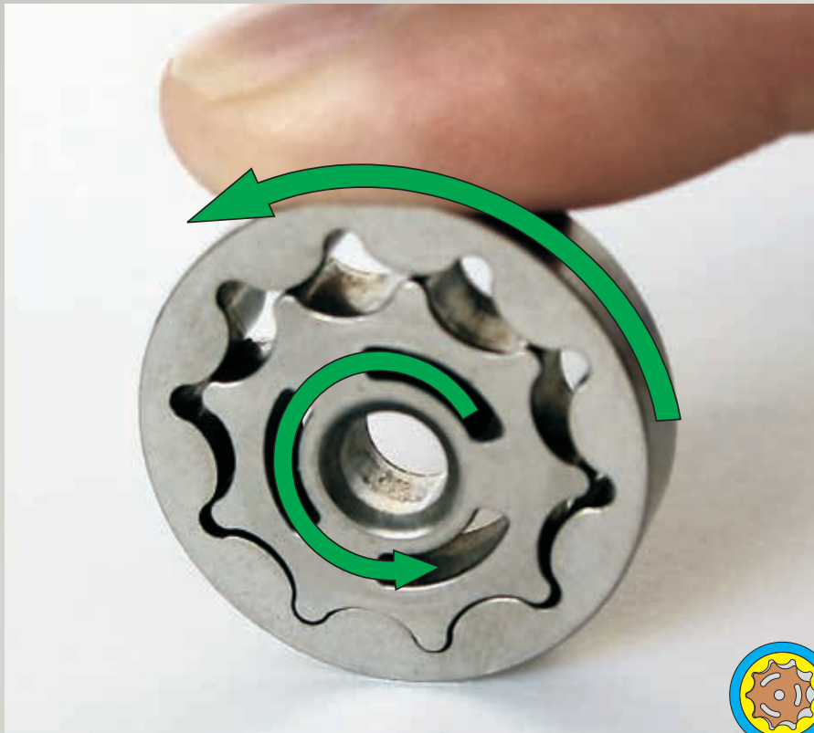
Fig. 52: The parts of a trochoidal pump system must mesh smoothly
