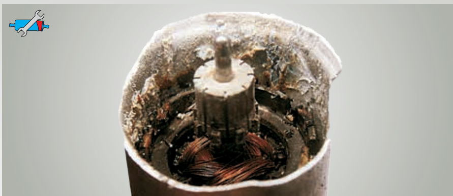
Fig. 16: Severely corroded electric fuel pump
