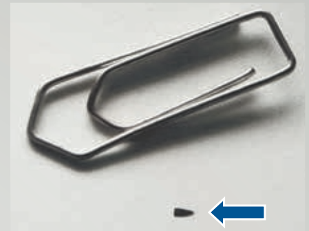
Fig. 27: Foreign body that caused the damage (shown with a paper clip to illustrate the size)
