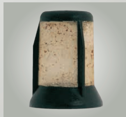
Fig. 23: Contaminated sieve filter of an E3T toothed ring pump
