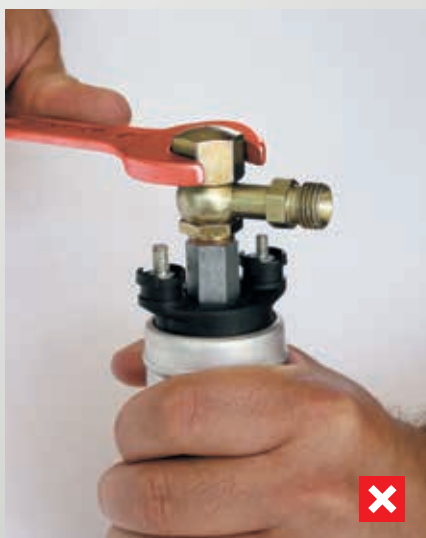
Fig. 70: Incorrect installation: Tightening without counter-tightening
