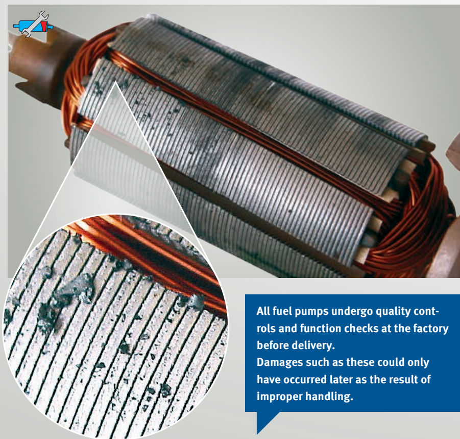
Fig. 80: Broken permanent magnet (stator)
