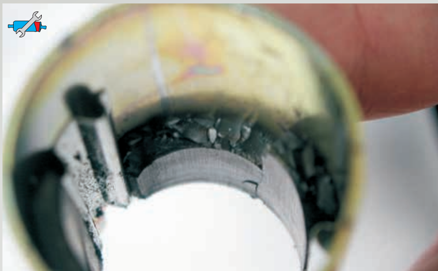
Fig. 80: Broken permanent magnet (stator)
