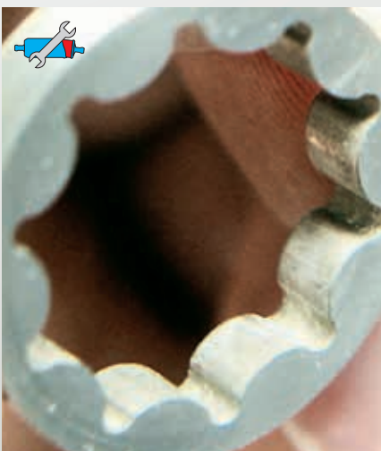
Fig. 51: Trochoidal toothed ring (with chalk deposits on left, new on right)
