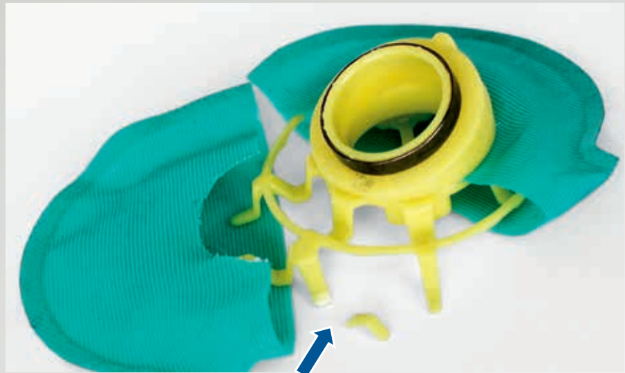
Fig. 76: Broken stiffening ribs in the filter of an in-tank pump
