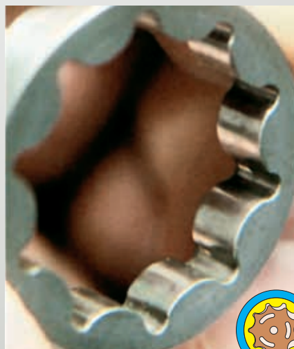
Fig. 51: Trochoidal toothed ring (with chalk deposits on left, new on right)
