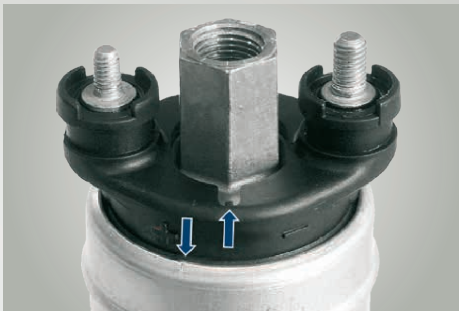
Fig. 69: Twisted pump cover
