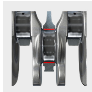
Fig. 3: Too large a rounding radius
