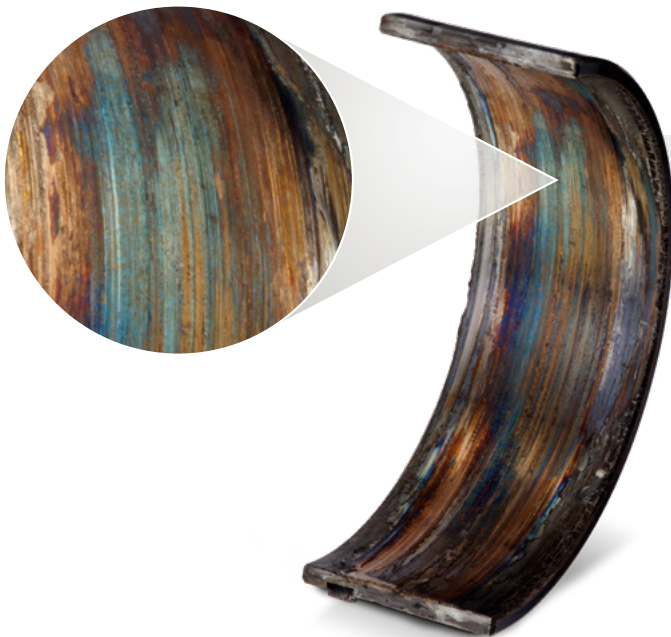
Cap-side conrod bearing shell steel-bronze composite with galvanic coating
