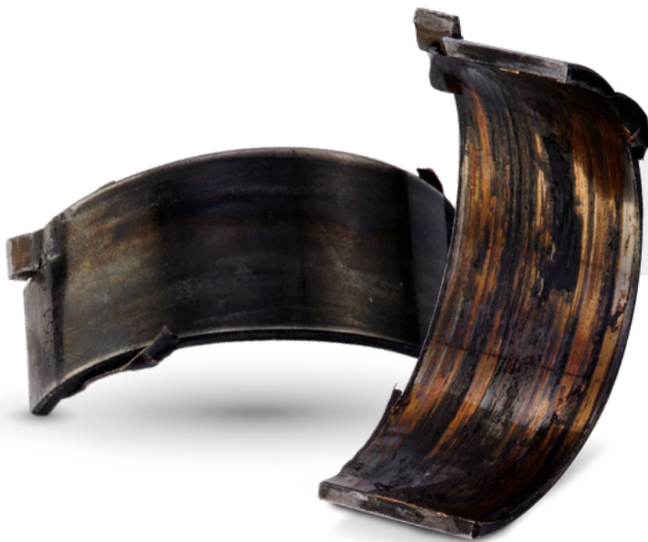
Rod-side conrod bearing shell steel-bronze composite with galvanic coating
