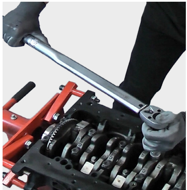
Tightening the bolts in accordance with the manufacturer's instructions
