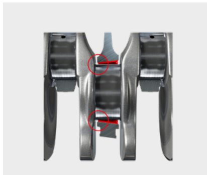
Fig. 2: Tapered bearing bore
