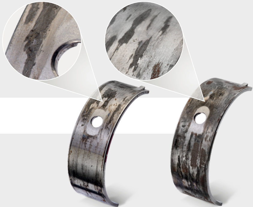
Fig. 2: Areas of torn-out material
