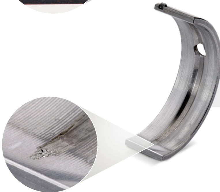
Upper main bearing shells steel-aluminium composite
