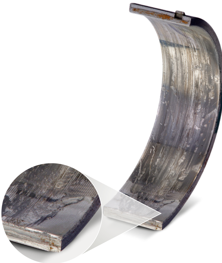
Lower main bearing shell steel-aluminium composite
