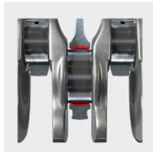
Fig. 2: Concave bearing bore
