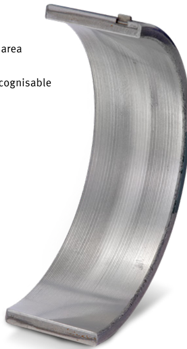
Lower main bearing shell steel-aluminium composite (without coating)
