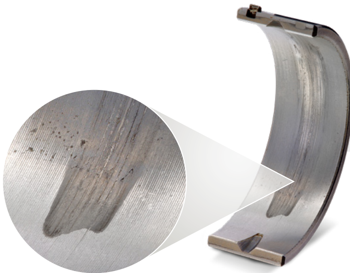
Lower main bearing shell steel-aluminium composite
