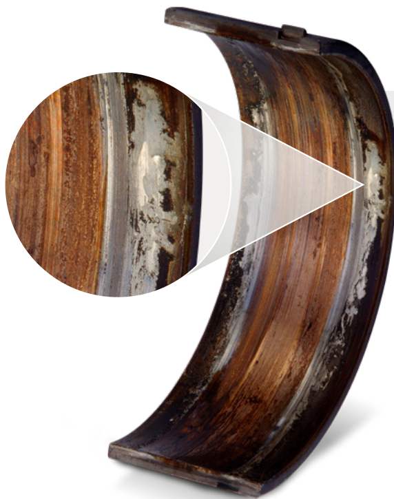
Cap-side conrod bearing shell steel-bronze composite with galvanic coating
