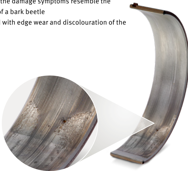
Rod-side conrod bearing shell steel-brass composite with sputter coating
