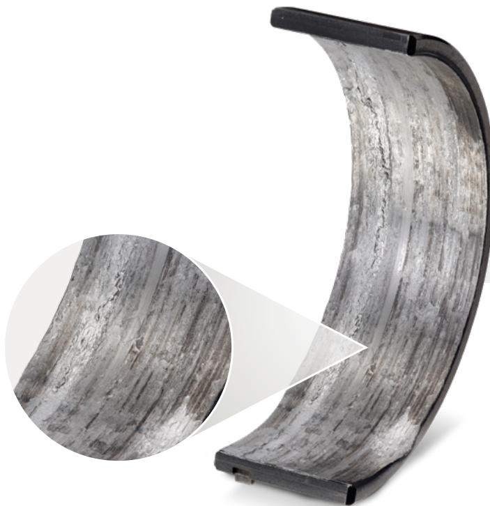
Lower main bearing shell steel-aluminium composite
