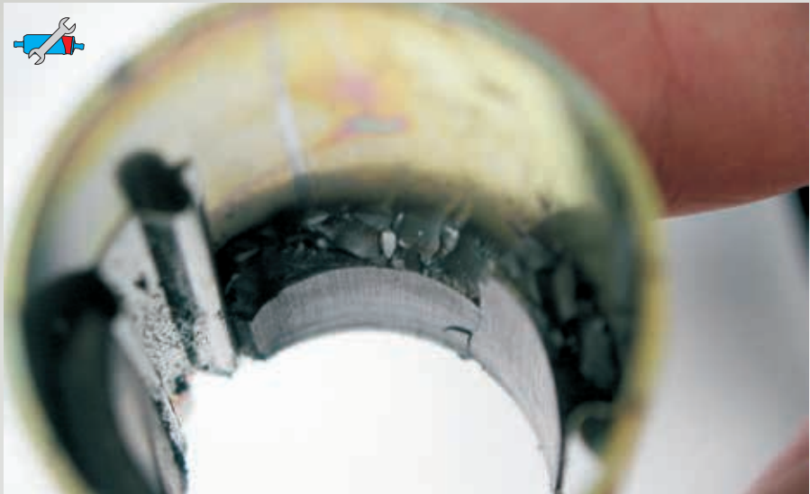
Abb. 80: zerbrochener Permanentmagnet (Stator)
