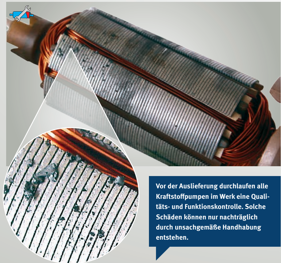
Abb. 80: zerbrochener Permanentmagnet (Stator)
