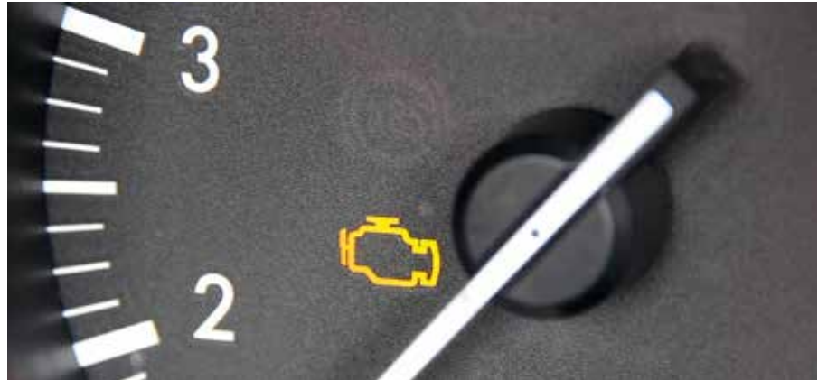
Fig. 6: malfunction indicator lamp (MIL)
