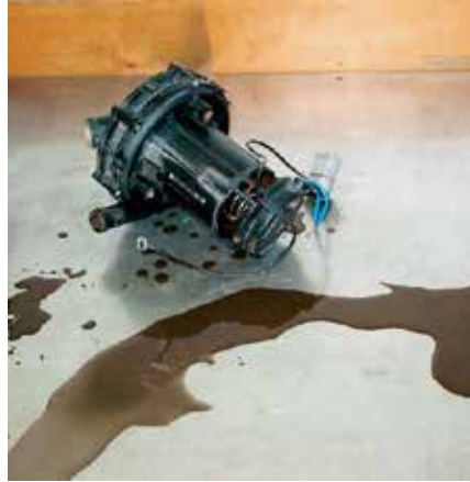
Fig. 28: condensate in the secondary air pump
