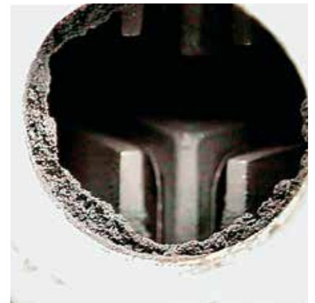
Fig. 31: deposits in the non-return valve
