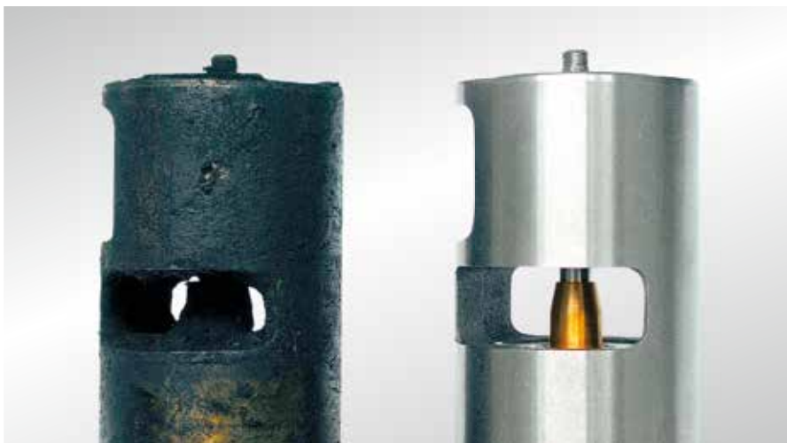
Fig. 38: EGR valve (diesel) with heavy deposits and new
