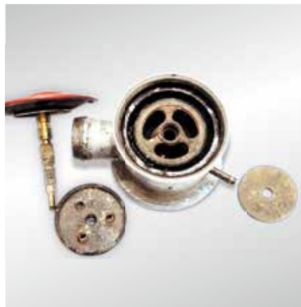
Fig. 30: cut-off secondary air valve – damage to the diaphragm and valve plate due to condensates
