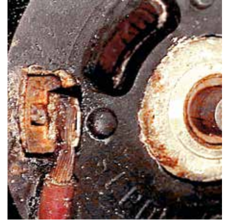
Fig. 29: secondary air pump – corroded electric connections
