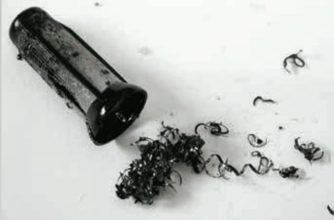
Fig. 29: Chips in the sieve filter Here, metal chips have entered the fuel tank during work on the fuel system. The sharp-edged chips have damaged the sieve filter. As a result, dirt can get into the pump and jam the pump system.
