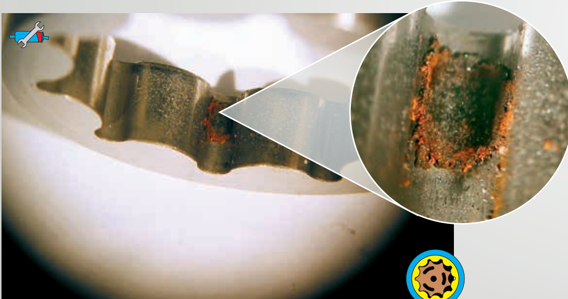
Fig. 47: Trochoidal toothed ring jammed by rust particles (microscopic image)
