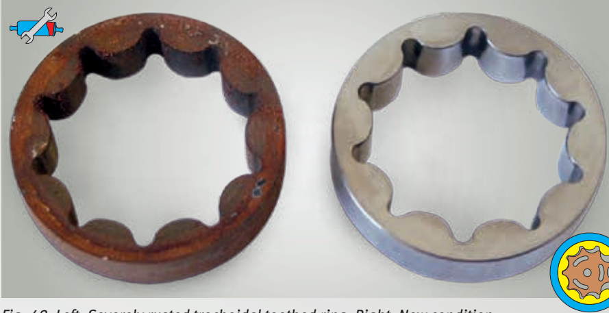
Fig. 48: Left: Severely rusted trochoidal toothed ring. Right: New condition
