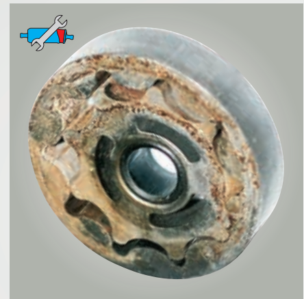
Fig. 53: For comparison: A rusty trochoidal pump system Here, nothing can move.
