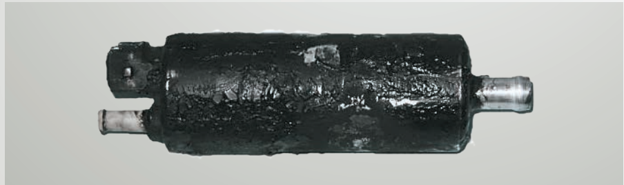
Fig. 65: In-line pump that was used as an in-tank pump
