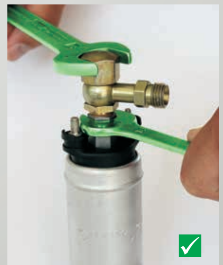
Fig. 71: Correct installation: The lower hex nut of the fuel pump must be counter-tightened
