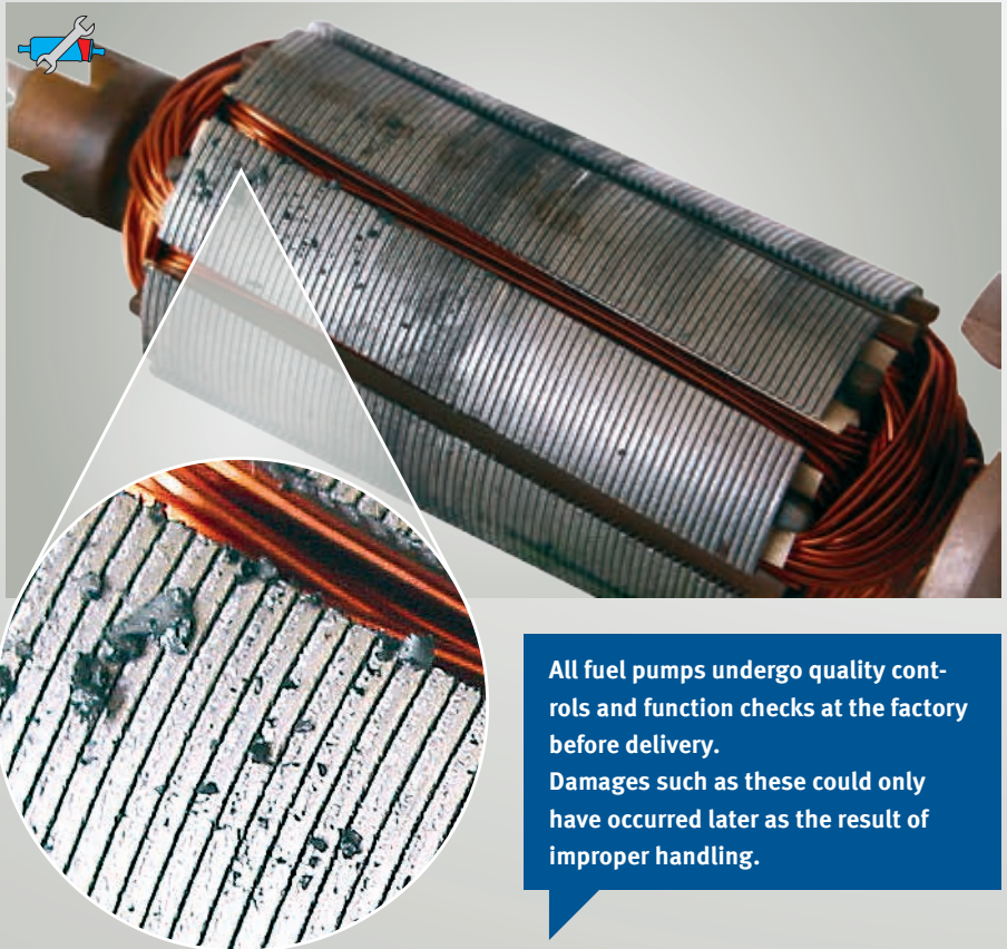
Fig. 80: Broken permanent magnet (stator)
