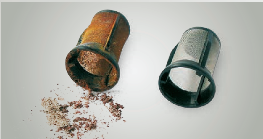
Fig. 41: Left: Sieve filter clogged by rust. Right: New sieve filter
