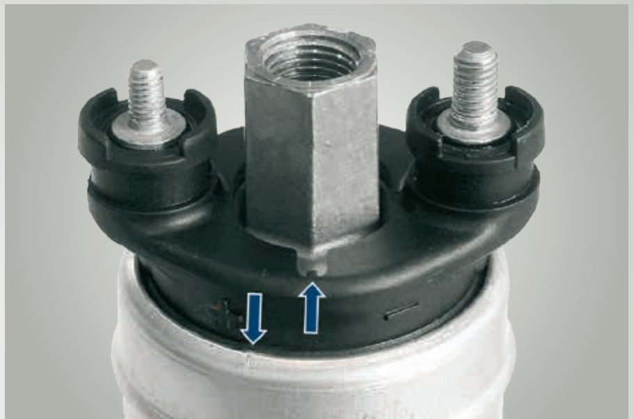
Fig. 69: Twisted pump cover There are markings on type E2T and E3T fuel pumps. These markings must be opposite one another. If they are not, the pump has been inexpertly handled and has been damaged as a result.
