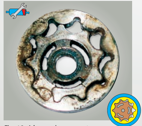
Fig. 19: A jammed pump system (trochoidal toothed ring) of an E3T toothed ring pump
