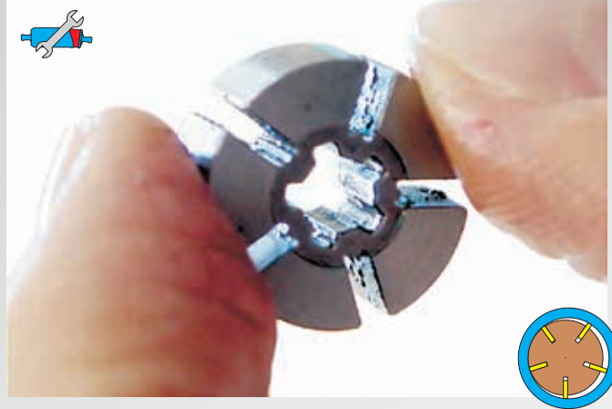
Fig. 30: Contaminated pump system of a vane-type pump The rotor is so clogged with dirt that the individual vanes (removed in this case) could no longer move. The pump still “runs”, but no longer supplies fuel.
