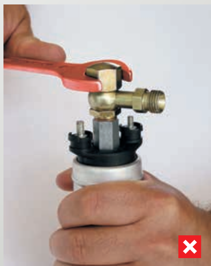
Fig. 70: Incorrect installation: Tightening without counter-tightening
