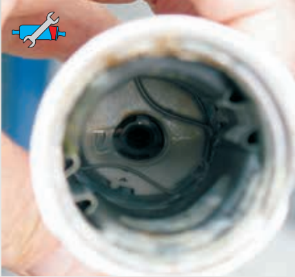
Fig. 44: Water in a fuel pump
