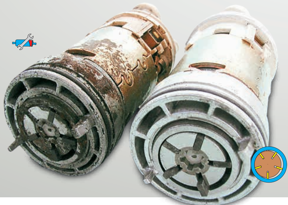
Fig. 36: Water damage to a vane-type pump On the right for the purpose of comparison is a fuel pump with comparable mileage, which has not been exposed to water.
