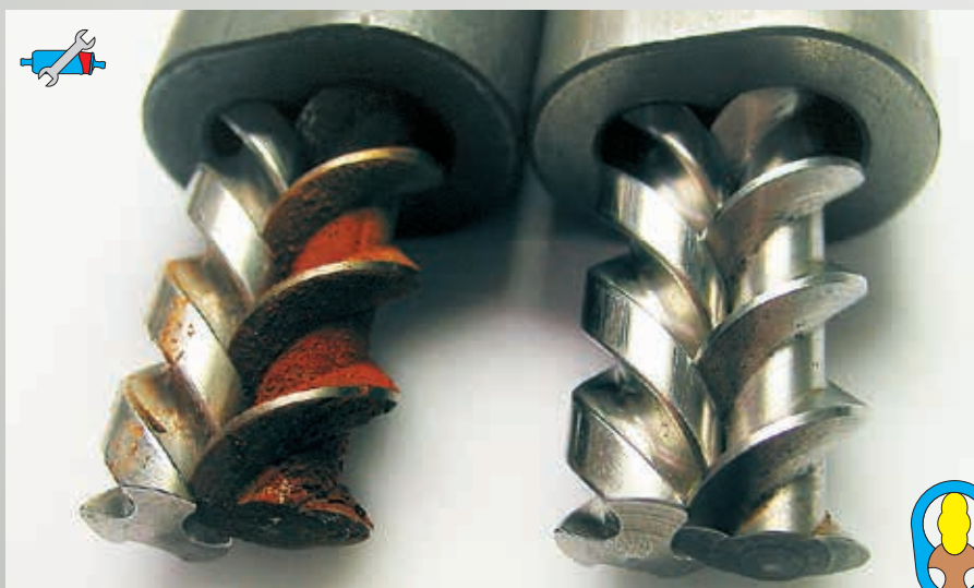
Fig. 54: Screw pump (rusty on left, new on right)
