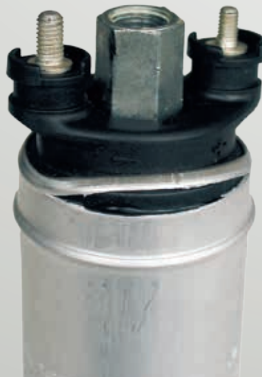
Fig. 1: Damage by force Damage is not always this obvious.
