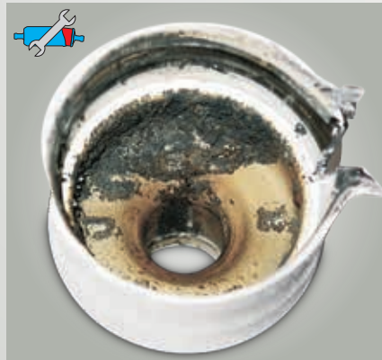
Fig. 18: A sectional view of the housing of an E3T toothed ring pump, clogged with debris
