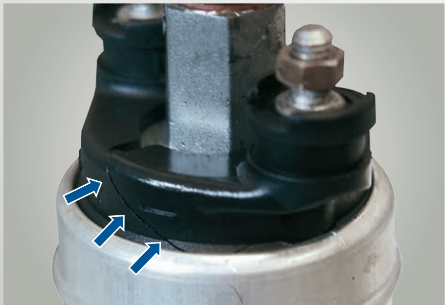
Fig. 73: Housing damaged by force
