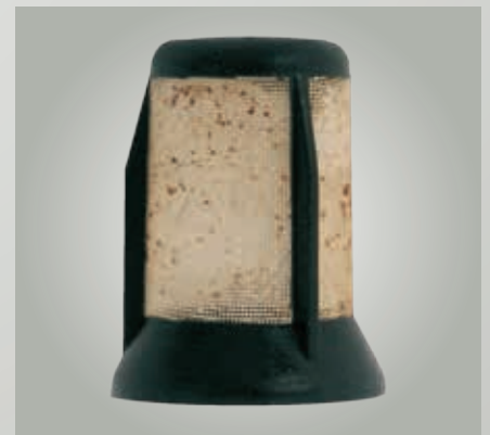
Fig. 23: Contaminated sieve filter of an E3T toothed ring pump
