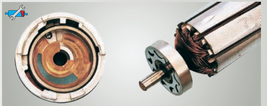
Fig. 38: For comparison: E3T toothed ring pump – In good condition despite a high mileage
