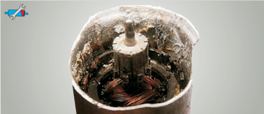
Fig. 16: Severely corroded electric fuel pump A view that repair shops don't generally have the opportunity to see. In many cases, it is only by opening the fuel pump that we can determine why a pump – seemingly intact from the outside – has failed.
