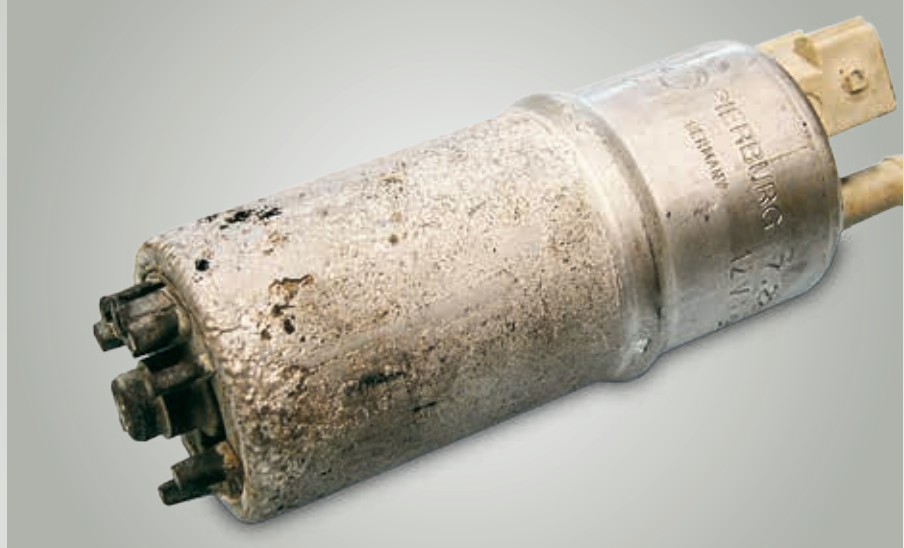
Fig. 72: Contact corrosion due to incorrect material combination
