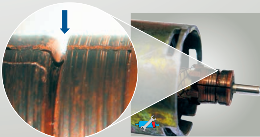
Fig. 63: Destroyed glide path of pole changer Here, after the carbon brushes had burnt off, the springs that press the carbon brushes against the pole changer “gouged” their way into the glide path.
