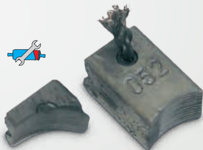
Fig. 62: Sliding contacts at approx. 9,500 miles Left: Prematurely worn. Right: Normal condition at this mileage
