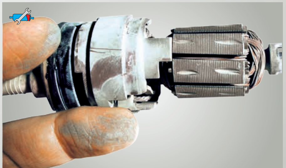
Fig. 56: Coating from poor-quality fuel
