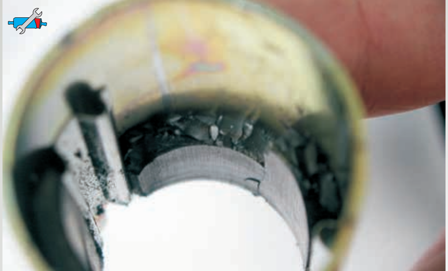
Fig. 80: Broken permanent magnet (stator)
