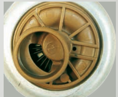
Fig. 35: For comparison: View inside the suction nozzle of a side-channel pump with undamaged impeller.
