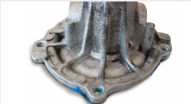
Bearing damage due to belt problems (rubber abrasion, particulate on the housing)
