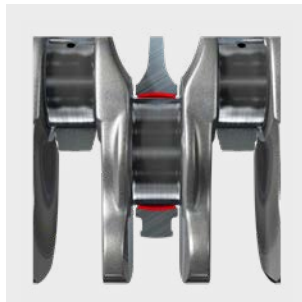
Fig. 2: Concave bearing bore
