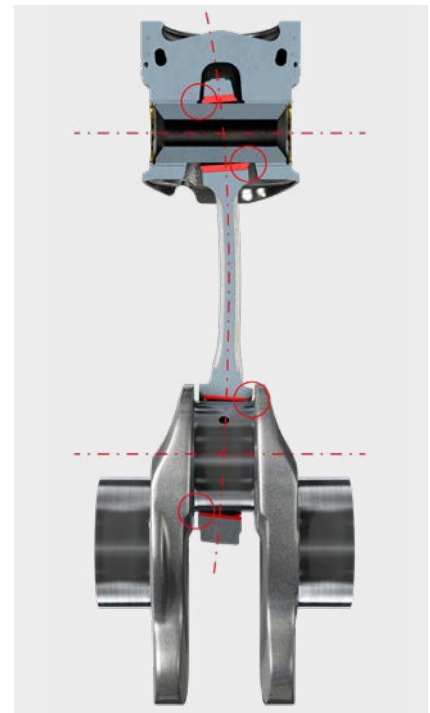
Fig. 2: „Maladjustment“ of the connecting rod
