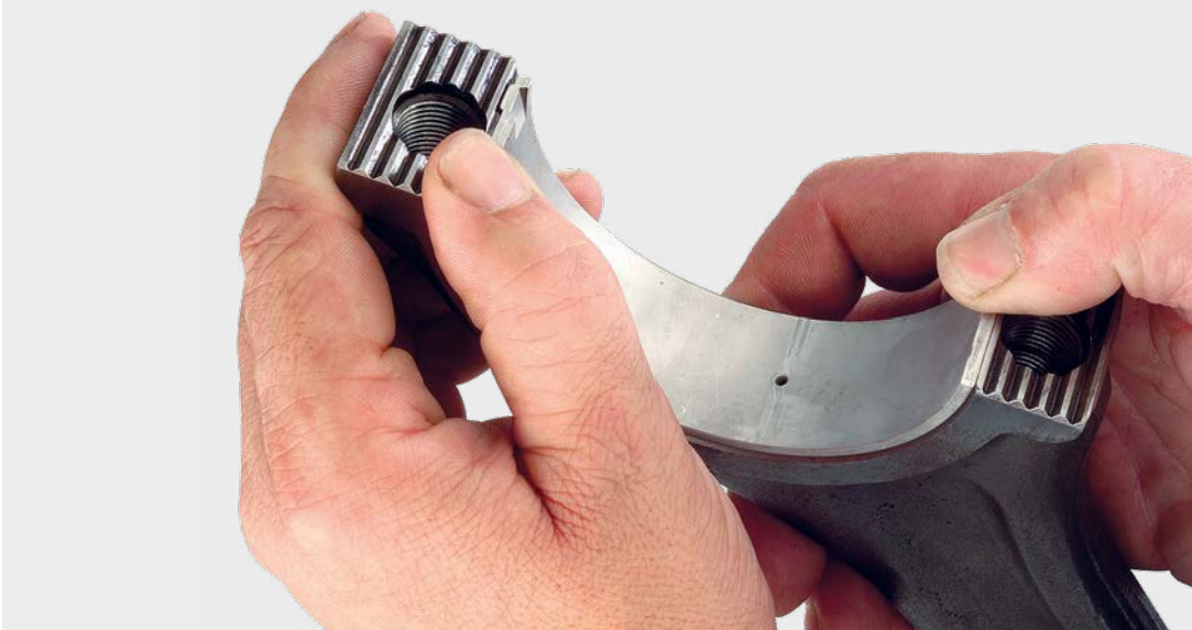
Documenting the seat and position of the bearing
