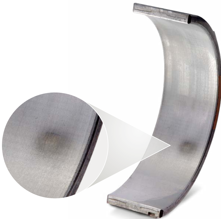
Lower main bearing shell steel-aluminium composite
