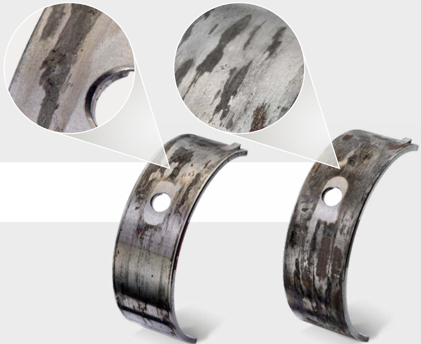
Fig. 2: Areas of torn-out material
