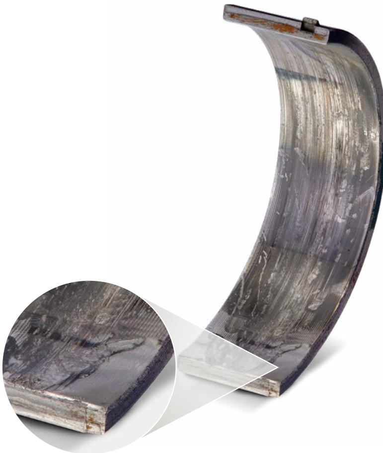
Lower main bearing shell steel-aluminium composite
