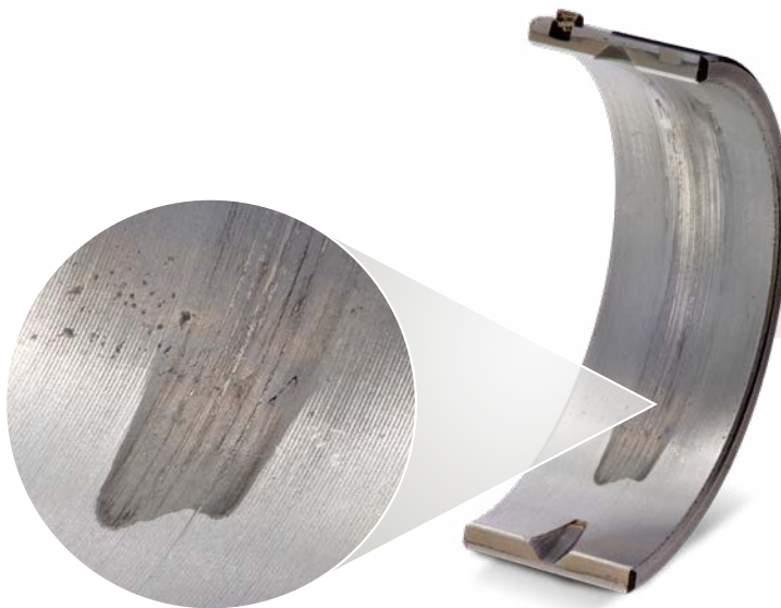
Lower main bearing shell steel-aluminium composite
