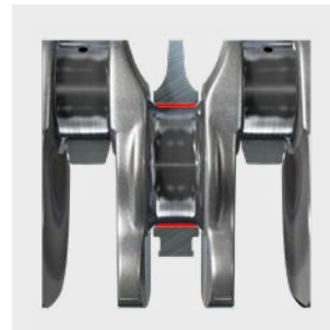
Fig. 3: Too large a rounding radius
