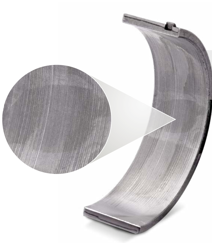
Lower main bearing shell steel-aluminium composite
