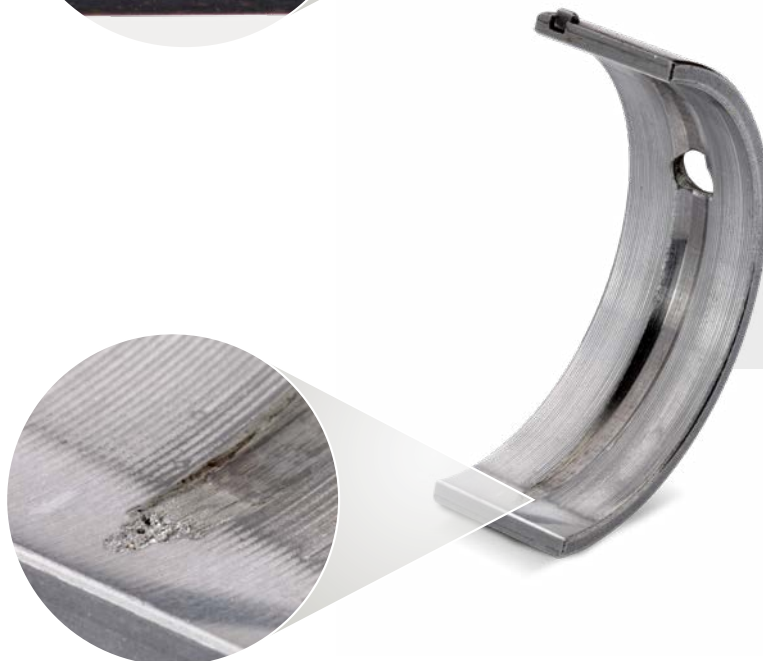
Upper main bearing shells steel-aluminium composite
