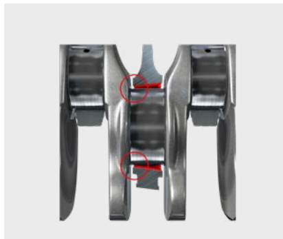
Fig. 2: Tapered bearing bore
