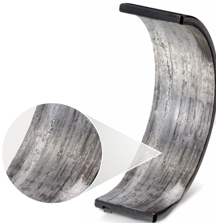
Lower main bearing shell steel-aluminium composite
