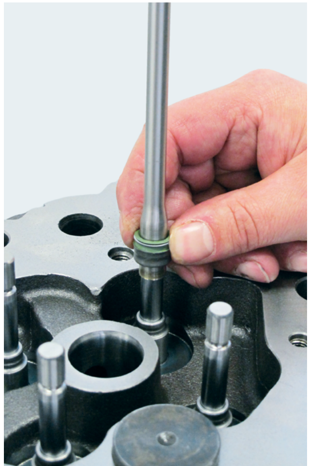
Fig. 2: Fitting a valve stem seal
