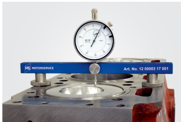
Fig. 2: Measurement of piston protrusion
