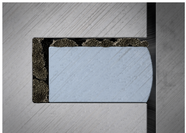
Fig. 3: Blocked piston rings
